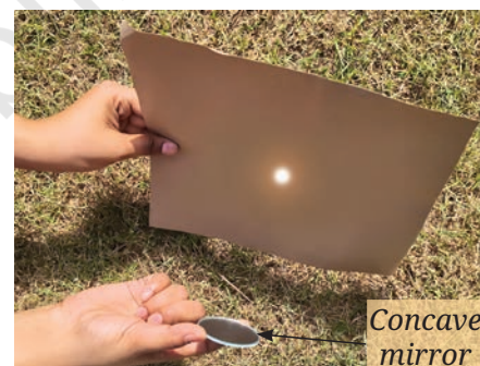
Fig. 10.12: Converging sunlight on paper using a concave mirror
